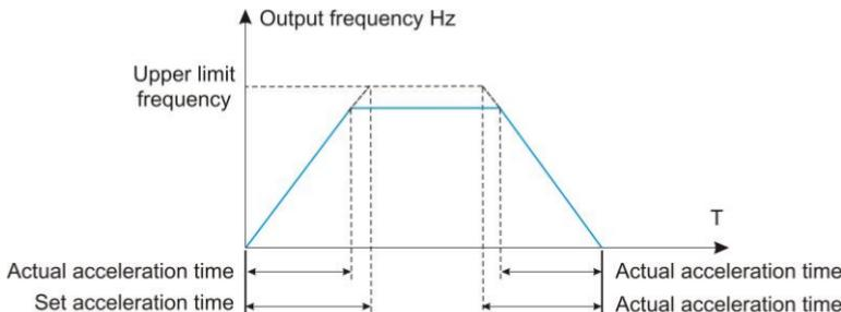
Fig. 6-1 Acceleration/Deceleration time
