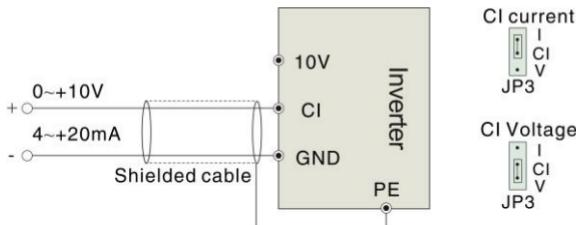
Fig. 3-10 CI terminal wiring
