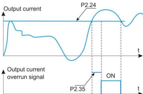
Fig. 6-14 Output current overrun detection
