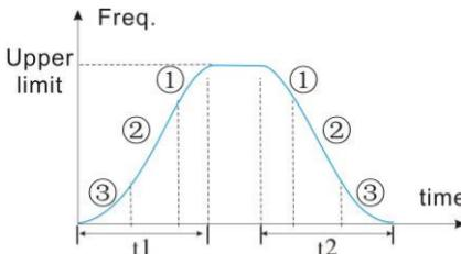
Fig. 6-04 S curve acceleration and deceleration
