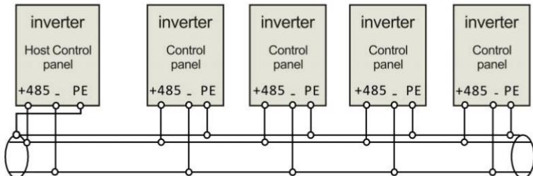
Fig. 3-15 Multi inverters communication
