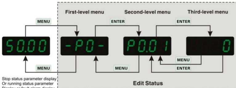
Fig.4-6 Operation panel programming display status
