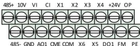
Fig. 3-8 Sequence diagram of control board terminal
