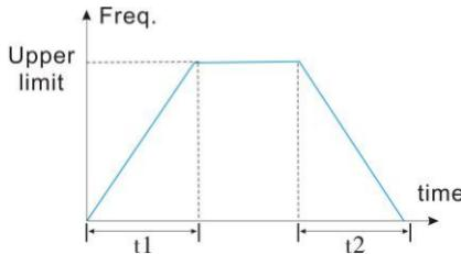
Fig. 6-03 Linear acceleration and deceleration
