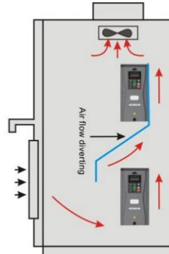
Figure 3-2 Mounting of multiple inverters
