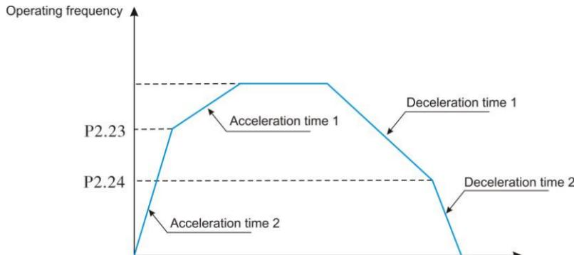
Fig. 6-12 Acceleration/deceleration switching
